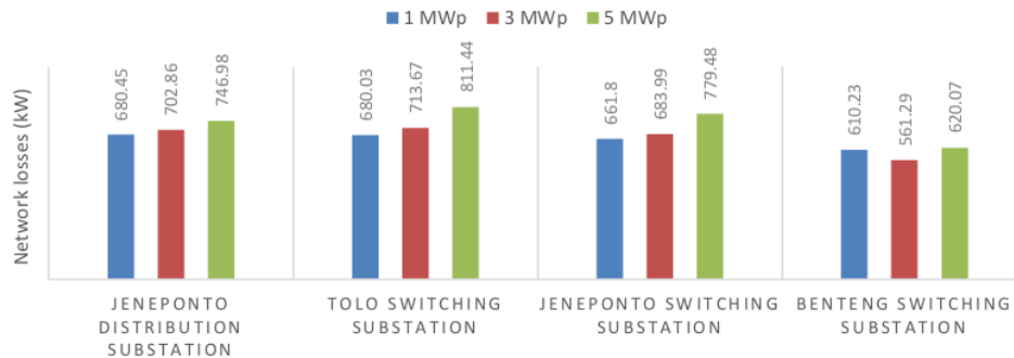
Figure 7. Total network losses for 1 MWp, 3 MWp and 5 MWp PV placement at different substations
